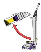
2 Remove clear bin and cyclone top from machine by lifting up until it releases.
